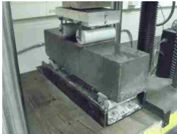
Figure 3.7. Beam Testing Apparatus
