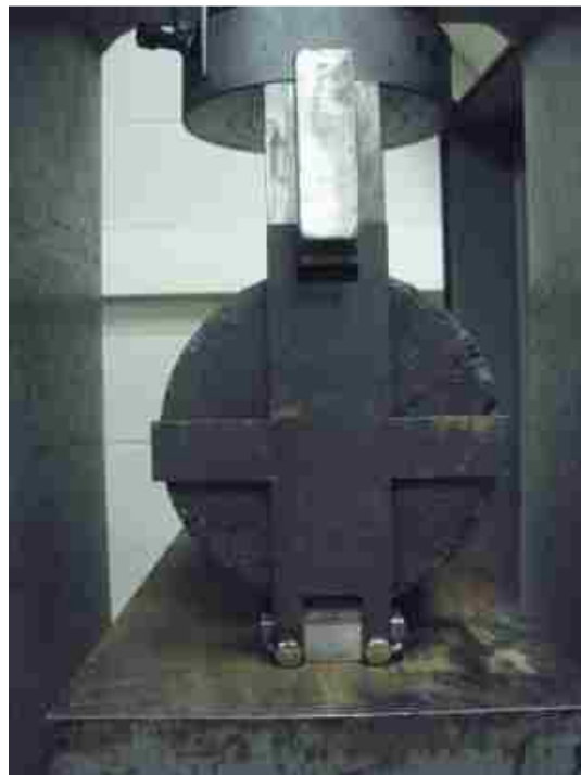
Figure 3.10. Splitting Tensile Testing Jig
